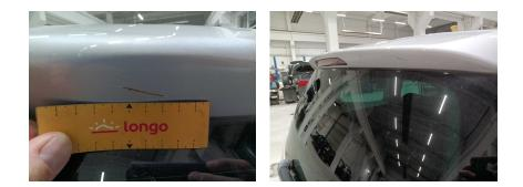
5. SIDE: Left and right side - visual damage / scratches
