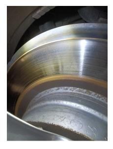
2. BRAKES: Front brake disc (both)
