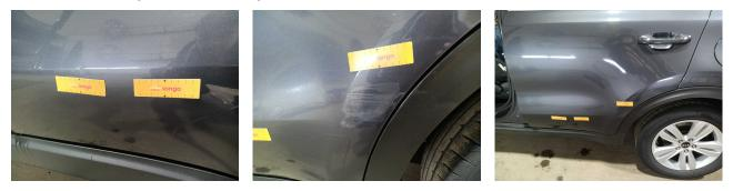
3. SIDE: Left and right side - visual damage / scratches
