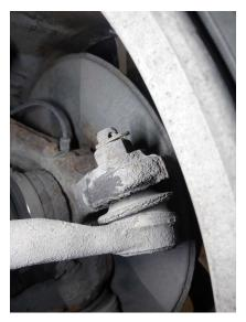
2. SUSPENSION: Ball joint - lower (both)
