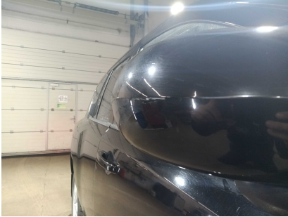
5. SIDE: Exterior mirrors - integrity of mirror itself and attachment to car
