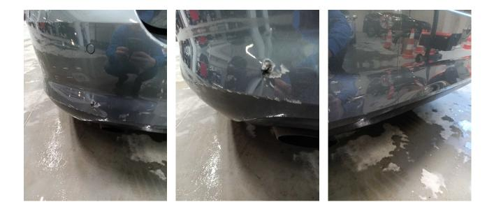
4. SIDE: Left and right side - visual damage / scratches
