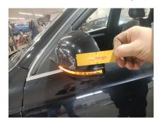
**6. SIDE:** Exterior mirrors - integrity of mirror itself and attachment to car
