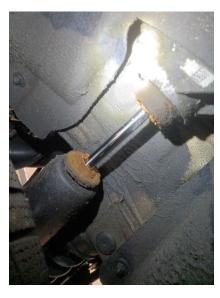
**2. SUSPENSION:** Strut top mounting (both)
