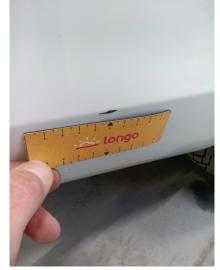
**6. SIDE:** Left and right side - visual damage / scratches
