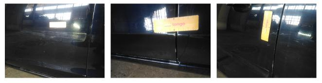
2. SIDE: Left and right side - visual damage / scratches
