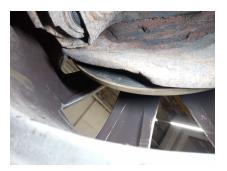
2. EXHAUST SYSTEM: Pipe - middle/silencer
