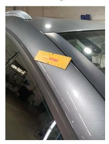
7. OTHER: Roof - visual damage (e.g., hail damage)
