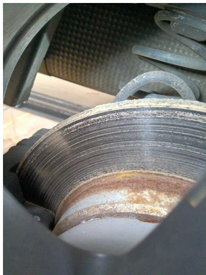
**2. BRAKES:** Front brake disc (both)
