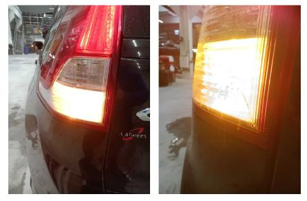
3. LIGHTS: Rear lights (brake, fog, indicator) - basic functioning, damage, color
