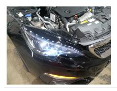
8. LIGHTS: Front lights (city, regular and full headlight, fog, indicator) - basic functioning, damage, color
