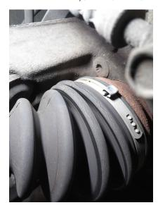
**3. FINAL DRIVE, SHAFT & AXLES:** Driveshaft seal - inner right
