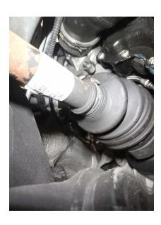
4. FINAL DRIVE, SHAFT & AXLES: Driveshaft joint - outer right
