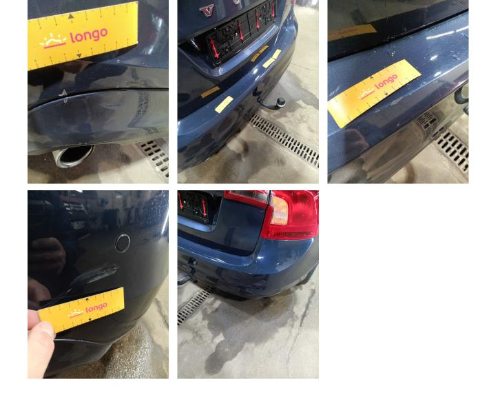
5. SIDE: Left and right side - visual damage / scratches
