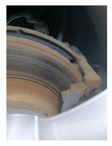
2. BRAKES: Front brake disc (both)
