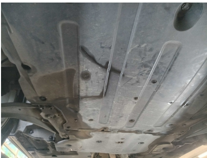
3. BODY - FRONT SECTION: Engine bottom cover damaged
