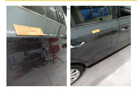
**2. SIDE:** Exterior mirrors - integrity of mirror itself and attachment to car
